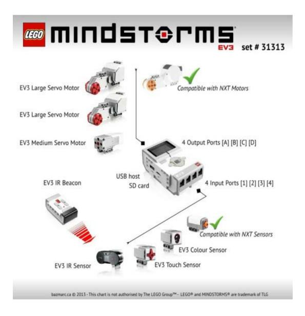
**Input Ports**- ports 1, 2, 3, 4 are used to connect sensors to the EV3 Brick.
