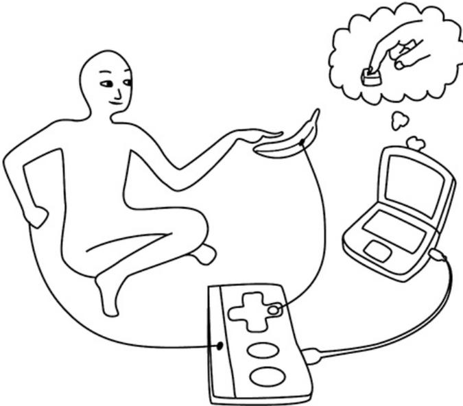
Alligator Clip two objects to the Makey Makey board. For example, you and a banana. When you touch the banana, you make a connection, and Makey Makey sends the computer a keyboard message. The computer just thinks Makey Makey is a regular keyboard (or mouse). Therefore it works with all programs and webpages, because all programs and webpages take keyboard and mouse input.
