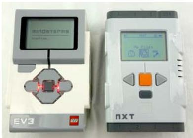
**EV3 Brick**- Serves as the control center and power station for the robot.
