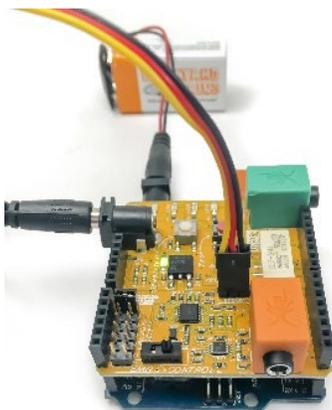
6. Plug the additional battery into the barrel connector on the blue Arduino board to power up the system.
