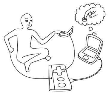
Alligator Clip two objects to the Makey Makey board. For example, you and a banana. When you touch the banana, you make a connection, and Makey Makey sends the computer a keyboard message. The computer just thinks Makey Makey is a regular keyboard (or mouse). Therefore it works with all programs and webpages, because all programs and webpages take keyboard and mouse input.
