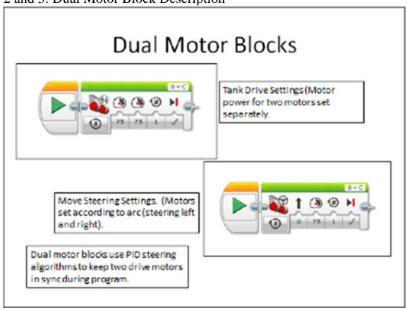
In this lesson we will use the Tank Drive Blocks to program our Robot to Drive in a Square. These lessons will work with any robot configured in the Tank Drive Setup similar to the Educator Robot.
