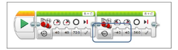
b. Now set the wheel degree rotation to 180 degrees. Remember, the degree rotation control how many degrees the wheels on the robot turn, not how far the robot turns. Download and test the program to note if the robot makes a 90 degree turn right or left. Adjust the degrees until the robot makes a 90 degree turn to the left.
