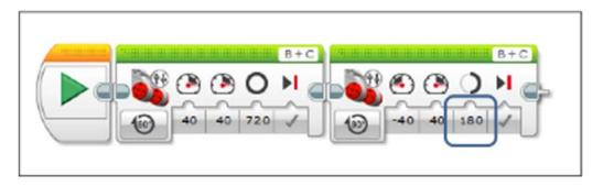
10. Now that we have one leg of the square complete, we can use a loop to complete the shape. Click on the orange flow control blocks and drag a loop block in front of the two motor blocks.
