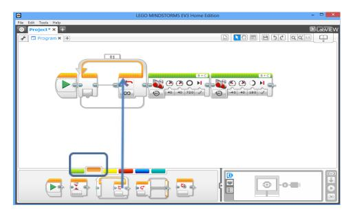
11. Drag the two motor blocks into the loop block.
