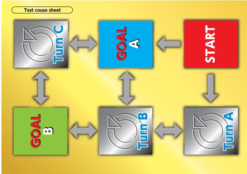
Let the robot run from the start to the goal. If you can make the robot run to the goal and stop within the goal square, you cleared the course. Use the data you recorded when you measured the performance of the robot in "2 Learn how the robot moves."
