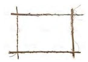
Create two rectangular frames, one for each side. For each frame, lay two 7-foot-long sticks parallel. attach one stick 5 inches from the tops of the two poles, another 10 inches from the bottoms, and the third in the middle. Next, nail two 60-inch-long sticks in an X shape on the bottom half for stability.
