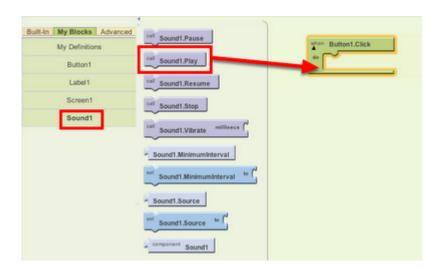
The purple and blue blocks are called **command** blocks, which are placed in the body of event handlers. When an event handler is executed, it runs the sequence of commands in its body. A command is a block that specifies an action to be performed (e.g., playing sound) when the event (e.g., pressing Button1) is triggered.
