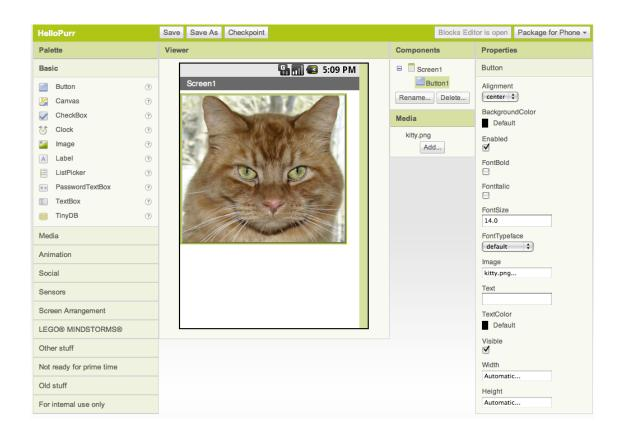
**Step 3.** From the **Basic** palette, drag and drop the **Label** component to the Viewer (#1), placing it below the picture of the kitty. It will appear under your list of components as Label 1.
